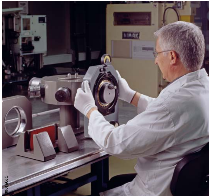
Figure 4 Positioning the enveloping circle gauge
