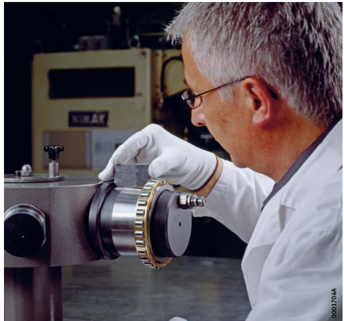
Figure 5 Measuring the spacing from the shaft shoulder
